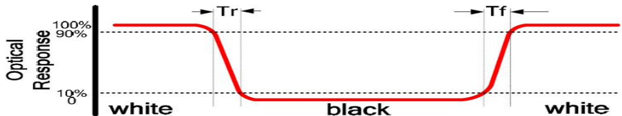
FIG2. Measuring method for Contrast ratio,surface luminance,Luminance uniformity,CIE(X,Y)chromaticity.
